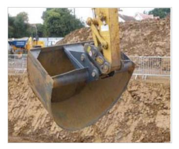
We designed an excavator bucket to produce a trench matching the shape of the pipe.
