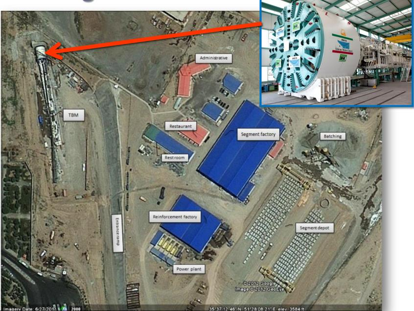
With a TBM and very Limited Space at the **Tunnel Face Just In Time** ls a Must...!
