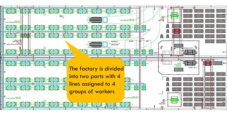
The segment factory is designed for 9 sets which form 9 complete rings...
